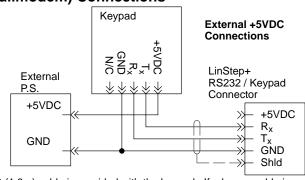
te: A 6ft (1.8m) cable is provided with the keypad. If a longer cable is to be used, an external +5VDC @ 500mA power supply is required.
